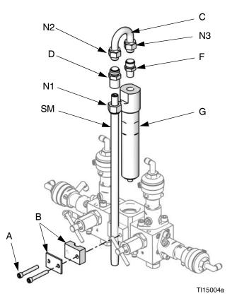
FIG. 8. Disassemble Integrator and Static Mixer
